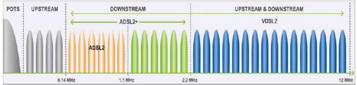
**Figure 2: VDSL2 Frequency Utilization**
